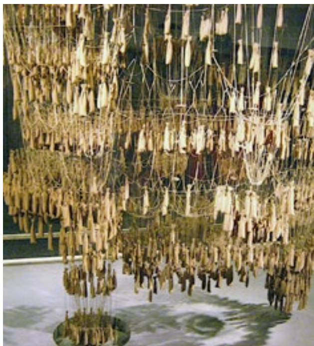
Figure-6: Gaudi's catenary design model for studying funicular forces
